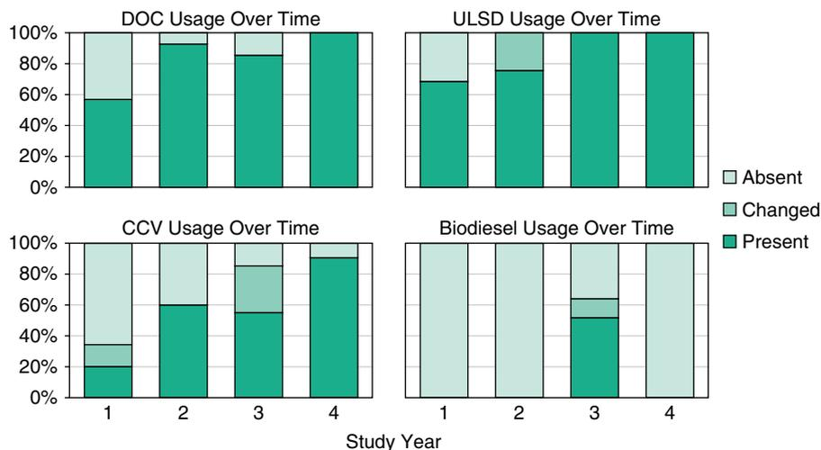
**Figure 1.** Clean air technologies and fuels over the 4-year study (defined as absent all year, changed during the year, or present all year). CCV = crankcase ventilation system; DOC = diesel oxidation catalyst; ULSD = ultralow-sulfur diesel.
